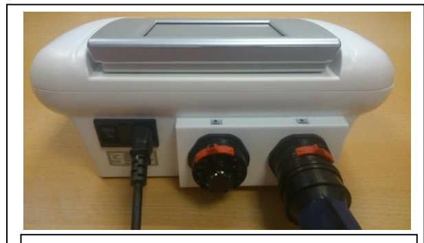
Example of connection 1 accessory: Sleeve (the other outlet remains free)
